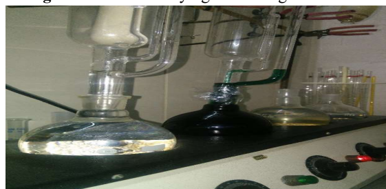
Figure 7:- Keratin Powder Extraction Unit (Soxhlet Extraction Unit)
