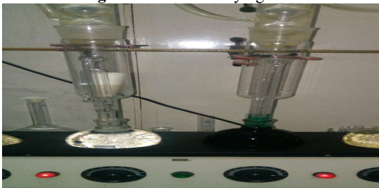
Figure 7:- Keratin Powder Extraction Unit (Soxhlet Extraction Unit)
